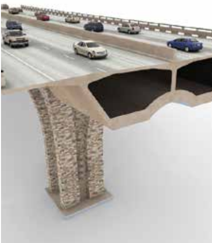
BRATTLEBORO. Cross-section of the new bridge being built over the West River.
